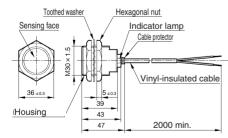
Vinyl-insulated cable (oil-resistant:  $0.5 \text{mm}^2, 20/0.18$  dia., 2-core), dia. 5.7. Cap color: blue.
