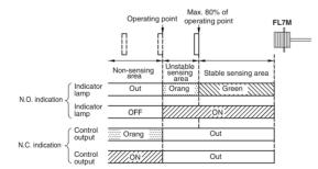
\*When the target object is made of a different material (such as aluminum, copper or stainless steel) from the standard target object (iron), the distance at which the indicator lamp changes color is shorter than the 80% maximum.
