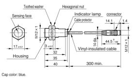
Hexagonal nut Toothed washer Indicator lamp connector Sensing face Cable protector 14.1 1.4 M18×1 ÷₩ dia.  $44.5_{-100}^{0}$ M12×1 4  $24{\scriptstyle\,\pm\,0.2}$ ±0.2 Vinyl-insulated cable 37 Housing 41 300 min. 45 Cap color: blue
